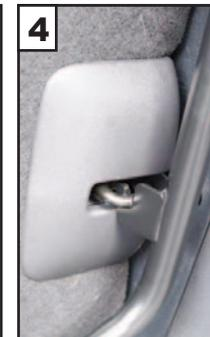
Centre the Dog Guard. Close the seats back. Secure the Dog Guard vertically by tightening the adjustable lower brackets 'B'.
