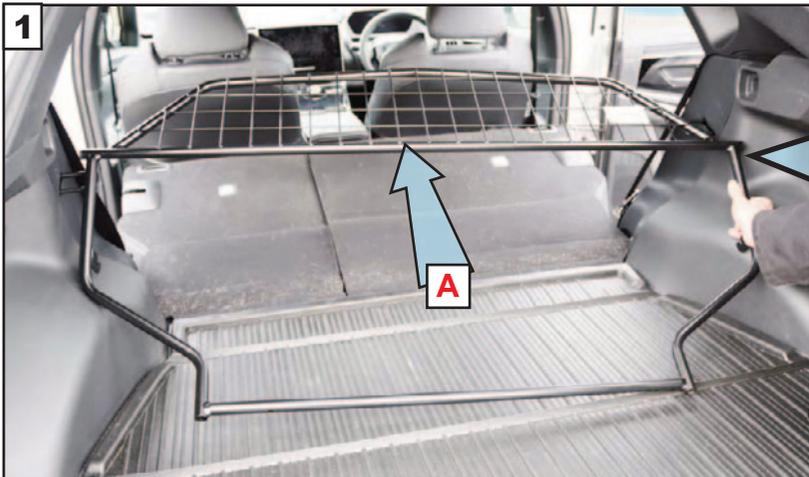
Drop the rear seats and offer in the Dog Guard. The mesh and badge need to be towards the rear of the car. The Dog Guard needs to be above seat locking bars as shown in the photo.
