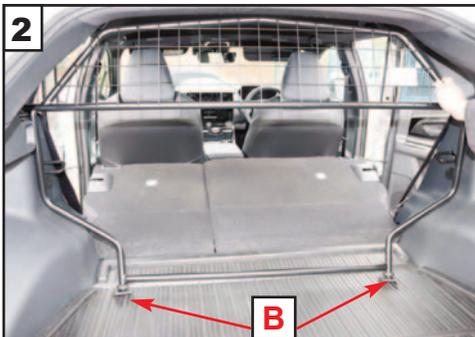
Insert the lower brackets 'B' into the open legs and then rotate the top of the Dog Guard upwards.
