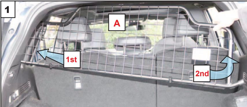
Insert the Dog Guard left hand side first. Then swing the right hand side into position. The Badge faces to the rear of the car
