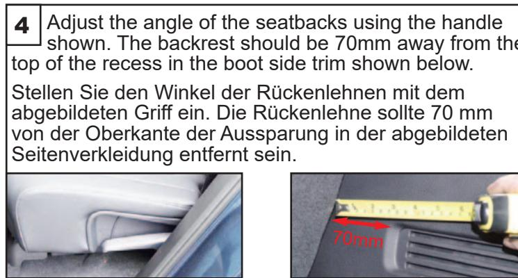
Adjust the angle of the seatbacks using the handle shown. The backrest should be 70mm away from the top of the recess in the boot side trim shown below.
