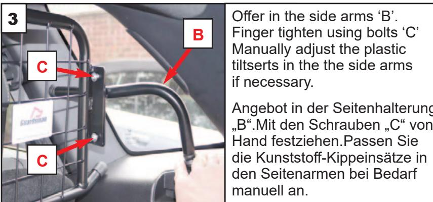
Offer in the side arms 'B'. Finger tighten using bolts 'C'. Manually adjust the plastic tiltsets in the the side arms if necessary.
