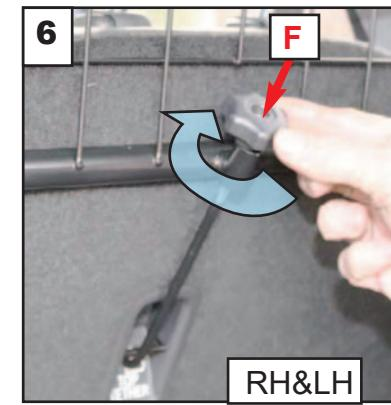
Tighten the handwheels 'F' until secure.
