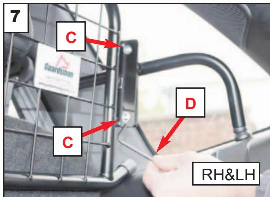
Then fully tighten both side arms 'B' using the Allen Key 'D'
