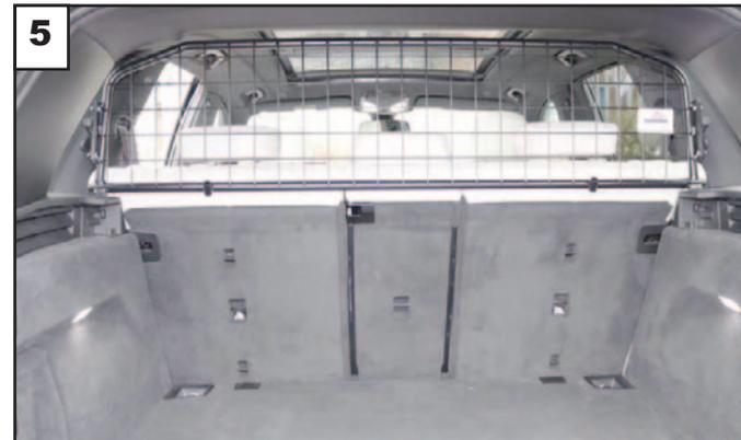
Hold the Dog Guard in position. Close the rear seats back into position.
