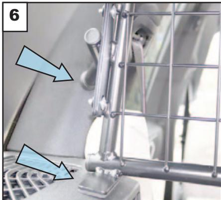
This is the required position for the side arms and lower brackets. Manually adjust the plastic tiltsets in the the side arms if necessary.
