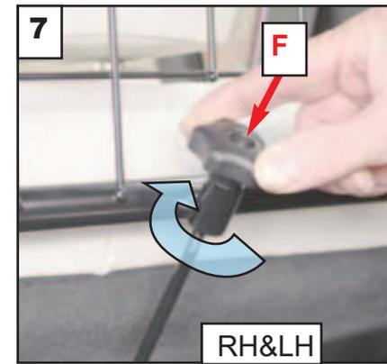
Tighten the hand-wheels 'F' until secure. Then fully tighten both side arms 'B'
