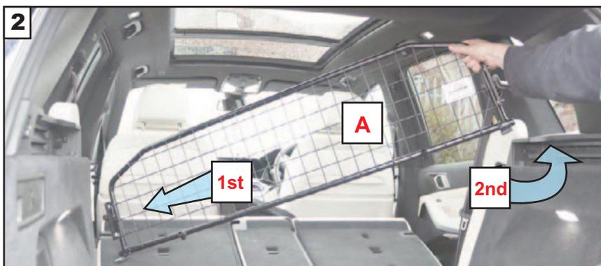
Drop the rear seats. Insert the Dog Guard left hand side first. Then swing the right hand side into position. The Badge faces to the rear of the car
