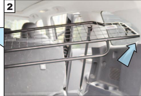
Push the Guard right into the window recess
