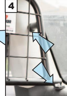
Position the side arm and lower bracket like this.
