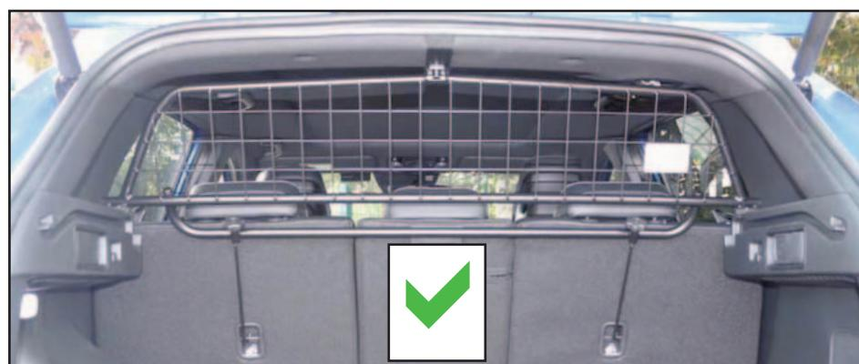
If you are fitting the Boot Divider do not fully tighten!
