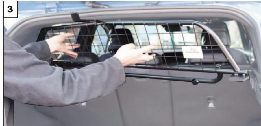
Insert the Dog Guard into position behind the rear seats. Put one end in and then swing the Guard around and upright. The Badge goes to the rear of the car.
