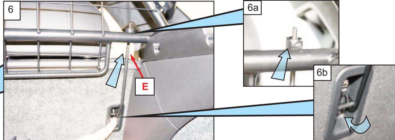
Take the securing Hook (F) and put it through the tubular guide in the lower rail of the Dog Guard. Then hook the securing Bar under the Child Seat Tether
