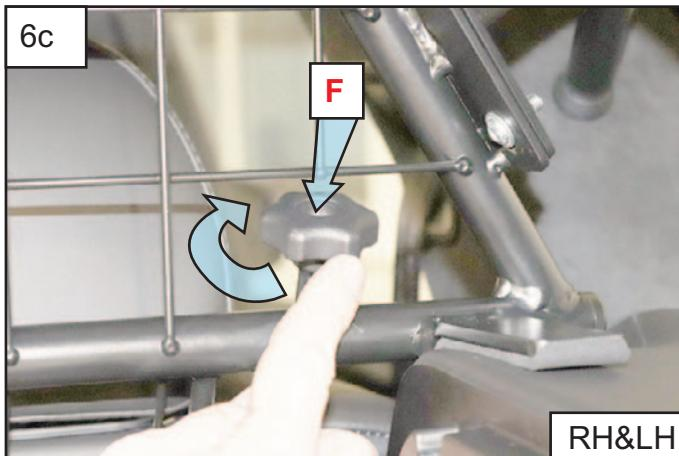
Partially secure with the Handwheels (F). If you are also installing a Boot Divider do it now.
