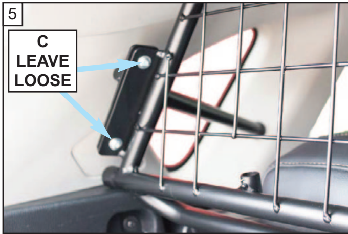
5 Position the Left Hand Side Arm (B) on the outside of the Dog Guard - Fix with the Bolts (C). Do not fully tighten
